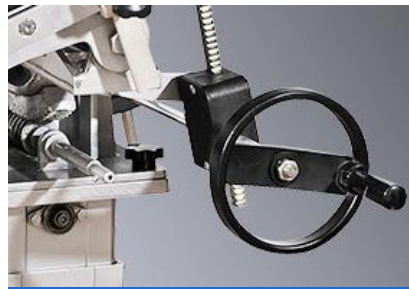
Manual wheel operation for Tren and Reverse Tren position
