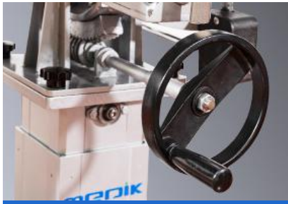
Manual wheel operation for tilting
